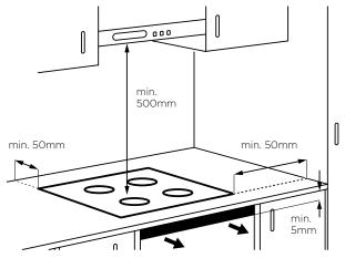
Make sure a ventilation space of 5mm directly below the benchtop is included in the installation and is kept free. The warranty does not cover functional failures caused by the lack of adequate ventilation
