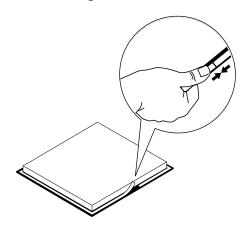
Assemble spring clips as shown, to support unit in benchtop.
