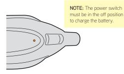
The charging light will illuminate continuously whilst the charger is connected.
