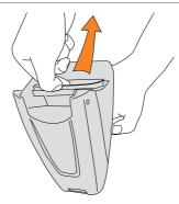
Whilst holding the dirt container over a bin, grasp the filter gently and pull out.
