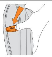
Press the filter removal button and pull dirt container from machine.
