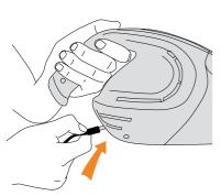
Plug charger into the mains and insert lead into back of machine. Initial charging time is 24 hours.
