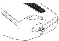
5. Place one open end of the bag material across the sealing strip and close lid.(Do not place edge of bag into vacuum channel when sealing bags)
