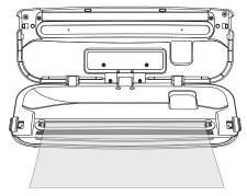
Close and lock lid by pushing the silver arrows on each side of the lid until fully closed.
