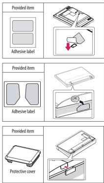
When installing the wall mounting bracket, it is recommended to cover the stand hole using tape, in order to prevent the influx of dust and insects. (Only UH65\*\*)
