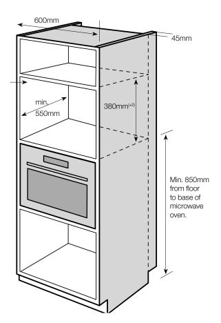
A 45mm ventilation gap must be left between the built-in cabinetry and wall with no back panelling on the cabinet housing the microwave oven.
