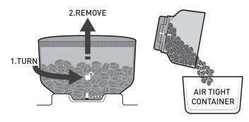
Wash the Bean Hopper in warm soapy water, then rinse & dry. Let the Bean Hopper stand to allow thorough air drying before replacing.
