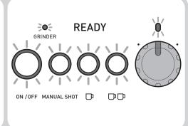
ON/OFF, EXTRACTION BUTTONS & DIAL LIGHTS all fully illuminated = Espresso Machine ready to use.
