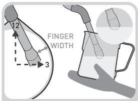
Insert Steam Wand Arm at 12 o'clock. Tip at 3 o'clock, finger width from edge and just below the surface of the milk.
