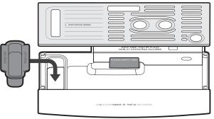
Place the Tamper in the detail provided on the Warming Plate.
