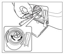
8. Make sure that the impeller of the pump can turn. If this does not occur, contact the service centre.
