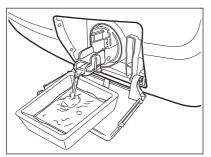
When the container is full of water, put the drainage duct back again and empty the container. Do steps 4 and 5 again and again until no more water flows out from the drain pump.
