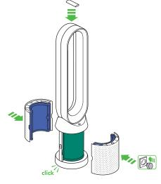
Position the shrouds onto the base and push gently until they click securely into place.
