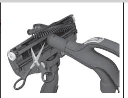
Pull out the brush roll and remove entangled threads by snipping them away with scissors. Use the hose handle to clean the nozzle. Refit in reverse order.
