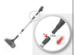
Attach the telescopic tube to the hose handle (to remove it, press the release button and pull the hose handle out).
