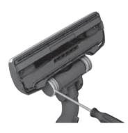
If the wheels are stuck, clean them by removing the wheel cap (only at the AeroPro nozzle) with a small screwdriver.
