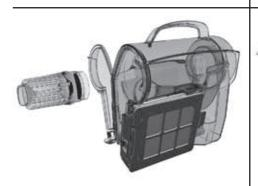
Remove the dust and fibres from filter. Clean the cone under the tap.
