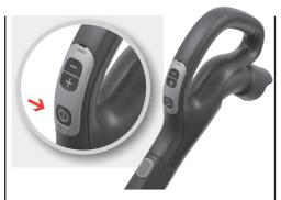
**Models with remote control** can also be operated by the (ON/OFF) () button on the handle.
