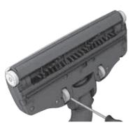
If the wheels are stuck, remove them carefully by using a small screwdriver.
