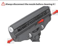
Open brush roll cover by pushing the latches. This will free the front wheels for cleaning.
