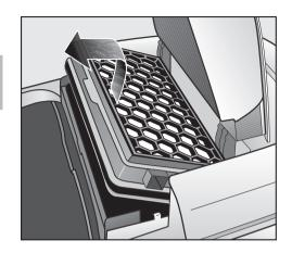
■ Replace with a new filter, and push it down into place.
