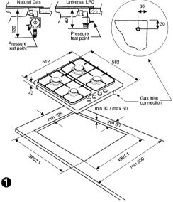
Before connecting the unit, check whether the local connection conditions (type of gas) are compatible with the unit's setting. Observe any special conditions imposed by local suppliers (utilities). The specifications of this cooktop are stated on the data label located on the bottom of the cooktop base.
