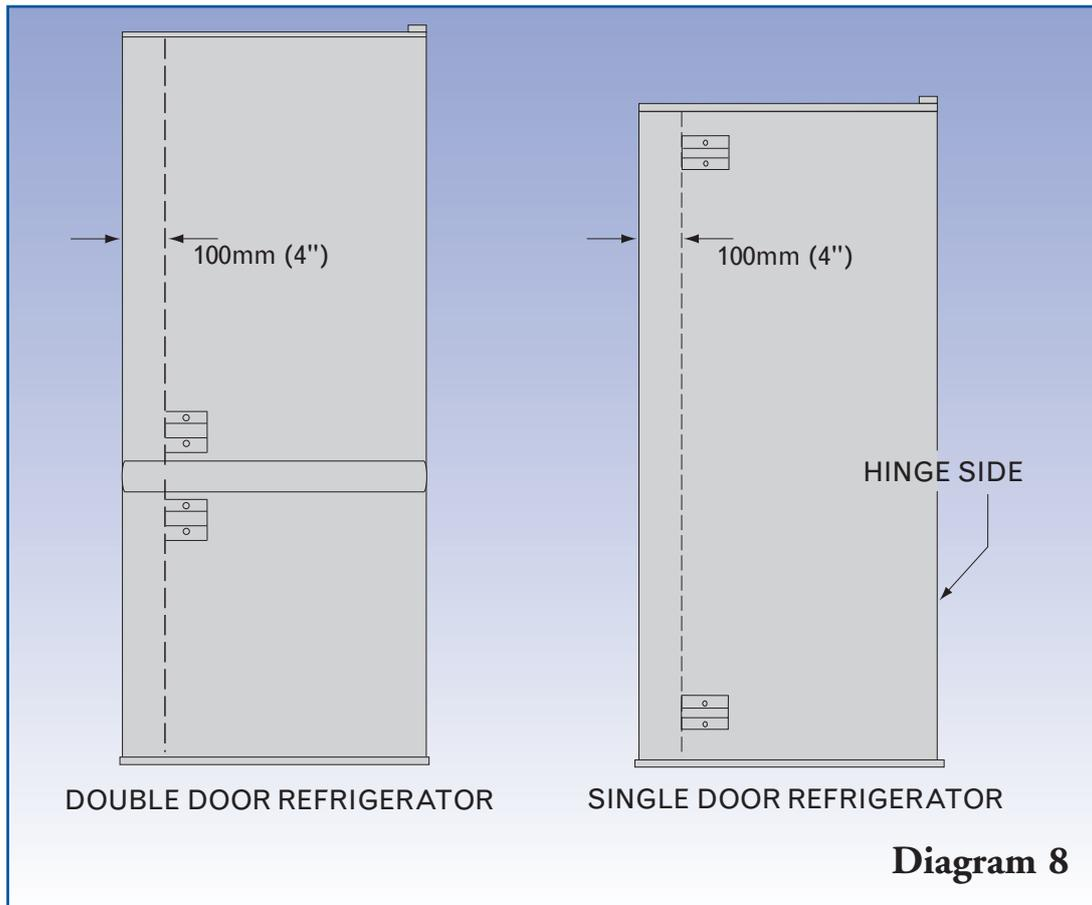
**Attach Slide bracket to Refrigerator Doors**
