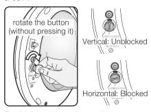
To disable this device and restore the possibility of closing the door, rotate the button anti-clockwise until the groove is vertical.
