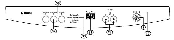
To operate, press the Off Timer button ③. The Off Timer indicator ③. will illuminate and the Combustion indicator ①. will be illuminated red to confirm that the heater will continue operation until the Delay 'off' time period has passed after which it will stop. The Delay Off time is 60 minutes. When this time has passed, the heater will automatically stop operation and the Off Timer indicator ③. will flash.
