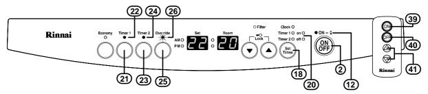
The heater must be between the finishing and starting times of a timer program for the Override to function to work. Either of the Timer indicators ② or ② will be illuminated and the Combustion indicator ③ is illuminated green when this is the case. If the Overrided button ② is pressed the Override indicator ③ will flash to show that the heater is now operating in override mode. The heater will now start and full manual control will now be available.
