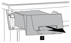
Push down the water tank's filler neck (1) and pull out it (2).
