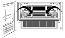
5. Use the handle to pull the heat exchanger out of the base and carry it horizontally to prevent any remaining water from spilling.
