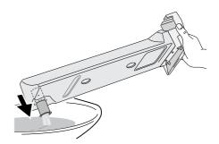
3. Push drainage pipe in and refit condensed water container.
