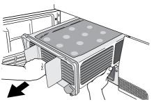
6. To empty the heat exchanger, hold vertically over a washing-up bowl.
