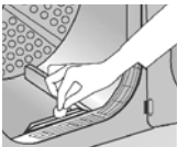
Fig.8 Cleaning the sensors
