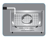
The submerged heating element system on the Avance™ Deep Fryer allows oil to be heated more effectively, and respond quickly to oil temperature changes.
