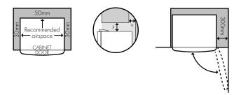
NOTE: Refrigerator doors on all models are designed to sit proud of cabinetry (not flush). The refrigerator should be placed against a wall of cabinetry and the clearance between the rear of the refrigerator and the wall should not be greater than 75mm.
