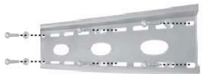
Fig. 2 - Attach the wall plate to the wall.
