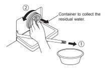
3 Remove any extraneous matter from the pump filter and cavity.
