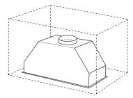
The PASC7801 FPX is a concealed canopy to be built into overhead cabinetry, whether it be wall, corner or island design
