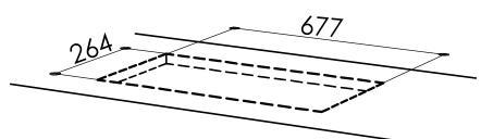
The PASC7801 FPX concealed canopy to be built into overhead cabinetry whether it be wall, corner or island design
