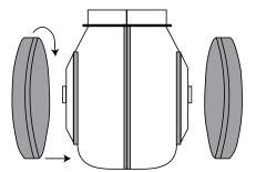
optional fitment of charcoal filters for recirculation installation
