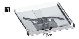
**STEP 1**Turn the filter anti-clockwise direction.
