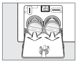
■ Remove the filters completely.
