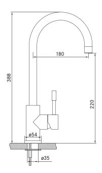
**PLEASE NOTE:** Large and heavy taps should ideally be mounted directly through the solid benchtop or fully supported from underneath. For all other swivel taps, we recommend the use of the Franke Tap Support Arm to provide additional support. Please ensure all Franke tapware is installed at a pressure of no greater than 500 kPa in accordance with AS/NZS3500 and insist that your plumber flushes all of the water supply lines before installing tapware. Failure to do so may void warranty.
