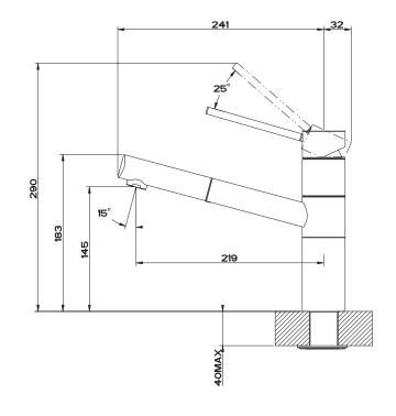
**PLEASE NOTE:** Large and heavy taps should ideally be mounted directly through the solid benchtop or fully supported from underneath. For all other swivel taps, we recommend the use of the Franke Tap Support Arm to provide additional support. Please ensure all Franke tapware is installed at a pressure of no greater than 500 kPa in accordance with AS/NZS3500 and insist that your plumber flushes all of the water supply lines before installing tapware. Failure to do so may void warranty.
