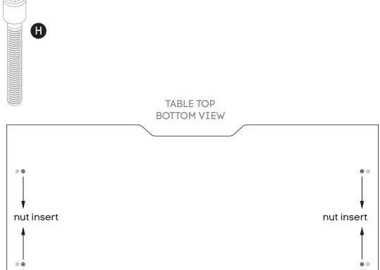
Place desktop ontop of frame - with cutout at the back of the desk. Nut inserts in top will align with plastic joiner brackets using M6x30MM **(H)** sockets attached top to frame.
