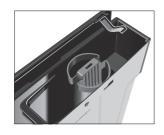
'Filter is being rinsed', the filter cartridge is rinsed. The water flows directly into the drip tray.
