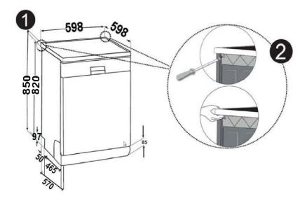
**Warning:** The stand part which we will settle our machine under it by removing its worktop has to be stable in such a way not to allow balance disorder.
