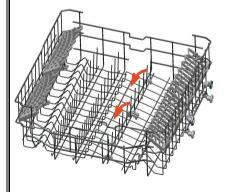
Foldable racks on the upper basket are designed in order to let you place big items easier such as pots, pans, etc. If requested, each part can be folded separately, or all of them can be folded and larger spaces can be obtained. You can use foldable racks by raising them upwards, or by folding down.
