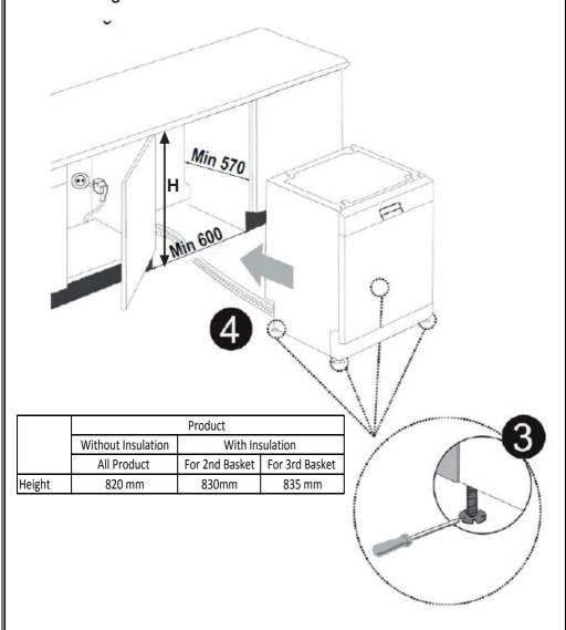
**Warning:** After removal of worktop, the machine should be placed in such a closed place of which dimensions are shown at fig.
