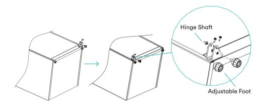
4. Remove the door upper cover, install the upper hinge sleeve, door signal line to the other side and install the door upper cover. Dismantle the right door stopper, sleeve pipe from the right bottom of door, insert the sleeve pipe into hinge hole of left bottom of door, and take out left door stopper from the accessory bag, and assemble it on left bottom of door, the right door stopper could be reserved for future use
