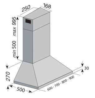
Model: IVX40 Canopy Hood Size: various Power standard: 10 Amp plug Ducting size: 150mm
