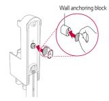
2 Use the remaining part of the tape to anchor the station to the wall before inserting the screw.
