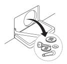
4 After cleaning, refit the pump filter and insert the drain tube plug.
