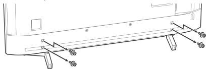
5 Install the TV to the Base. Refer to "5" of Installation Guide and "Installing the TV to the Wall" of Operating Instructions supplied with the Wall-Mount Bracket.
