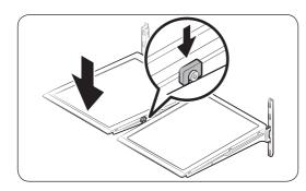
• To remove a shelf, fully open the corresponding door. Hold the front of the shelf, and then gently lift up and slide out.
