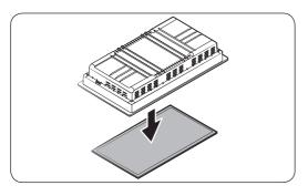
**5.** Turn over the basket to remove the metal cooling plate.
