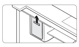
**1.** While grabbing the handle of the ice bucket, slightly lift up the bucket, and then remove it to the front.
