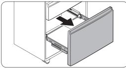
**4.** While holding the upper area of the drawer front of the freezer, slide out all the way to remove the freezer drawer from the rail assembly.
