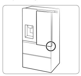
**1.** Check the height difference between the doors, and then raise and hold the door with the lower height.
