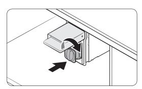
**3.** Insert a new filter cartridge. Use only Samsung-provided or approved filters.
