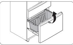
**2.** Pull up to remove the **lower basket** from the rail assembly.
