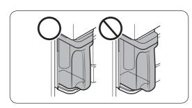
• To prevent the water tank from tipping over or leaking, make sure the water tank fits in the water tank holder.
