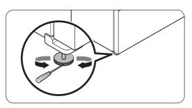
• To adjust the height on one side: Insert a flat-head screwdriver into a notch in the leveller on that side. (left or right) Turn the leveller clockwise to raise the refrigerator. Turn it counterclockwise to lower. Repeat on the other side.
