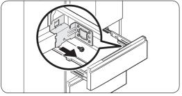
**4.** Remove the hex-head bolt from each side using a socket wrench (10 mm) or a screwdriver.
