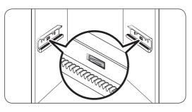
**3.** Press down the hooks to unlock the rail assembly.
