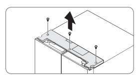
**1.** With the door opened, remove the screws from the **top cover**.
