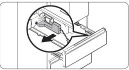
**2.** Remove the wire cover with harness using a flat-head screwdriver.
