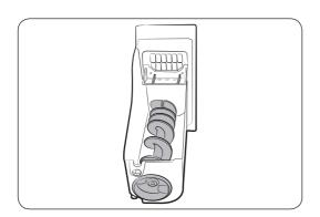
If the ice bucket is not firmly inserted, turn the ice screw 90 degrees, and then try again.
