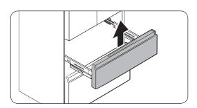
**5.** Lift up to remove the **drawer front of the CoolSelect+ (FlexZone)** from the rail assembly.
