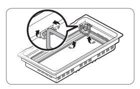
**3.** As the divider has the width and length bars, push the lower part of each bar inward to unlock. See the figures for details.
