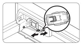
**3.** Press the locking tab to disconnect the wire connector.
