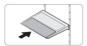
To remove, slide up the front of the shelf so that it folds. Then gently lift up and pull out. To reinsert, place the shelf on the angled frame in the main unit, and then, press down to unfold.
