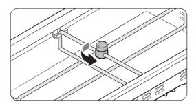
You can change the divider position. To do this, unlock the divider by turning the divider dial counter clockwise. Then, move the width and height bars as appropriate. When done, turn the dial clockwise to lock the divider.
