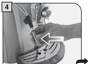
Remove the outer sleeve of the hot water / steam wand; thoroughly rinse it under running water, then re-insert it.
