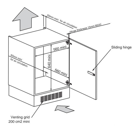
Overall depth: 555 mm including door and sliding hinge
