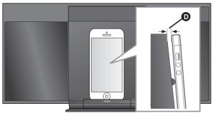
• There will be a gap between this unit's sliding door and the connected device.
