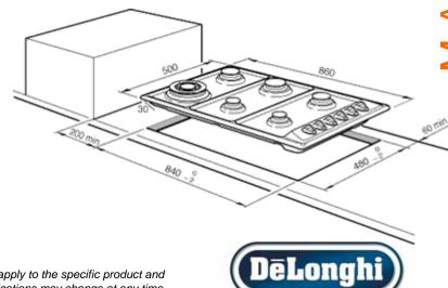
The product dimensions and specifications on this page apply to the specific product and model at the time of issue. These dimensions and specifications may change at any time. \*Diagrams are a guide only. Final fittings should be made with actual product.
