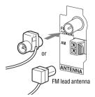
Keep the antenna away from the speaker cords and the power cord to avoid picking up noise.
