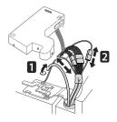
4 Rotate the hinge lever counterclockwise
