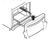
5 With both hands, flex the center bar enough to allow the gears on both ends to release from the track.
