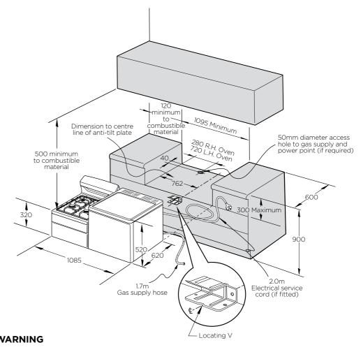
In order to avoid accidental tipping of the appliance (for example, by a child climbing onto the open oven door), the anti-tilt plate and stabilizing bolt MUST be installed.
