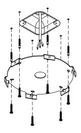
**2** • Feed the power cable from the drop-rod into the ceiling rose cover.
