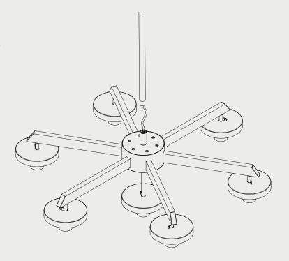
**3** Raise the pendant towards the ceiling and make the electrical connections.
