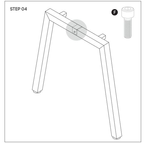
Using Allen Key provided, attach M8x20MM Socket head (F)-screw socket half way into leg for both legs (B)
