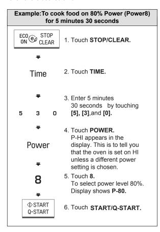
When cooking is complete, four short tones will sound. The word **End** shows in the display window. Then the oven shuts itself off.
