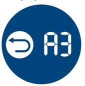
With advanced AeraSense technology, the filter lifetime is accurately calculated based on indoor pollution level, air flow and operation time. Healthy air protect alert lets you know promptly when it is time to replace the filter. If the filter is not replaced promptly, the appliance stops functioning to avoid running with no effect since filter not effective. So you are assured of healthy air always.
