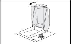
4. Lift the lid upwards to remove it.
