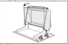
3. Lift the lid upwards to remove it.
