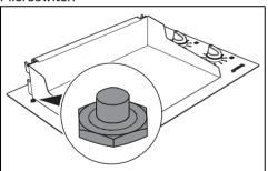
It detects whether the appliance's lid is open or closed, useful for adjusting settings and ensuring the ideal temperature on the grill.
