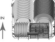
It is suggested that large items, and items thar are most difficult to clean, are placed in the lower basket — eg pots, pans, lids, serving dishes etc. It is preferable to place serving dishes and lids on the side of the racks to avoid blocking rotation of the top spray arm.
