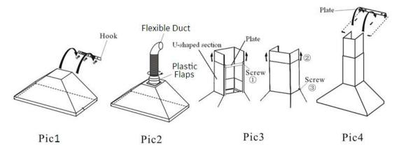
Note: Fix the Canopy with two 30mm safety screws. The two safety screw holes are positioned on the back casing (refer to Pic 5).
