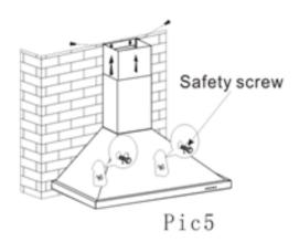
Warning: Failure to install the screws or fixing device in accordance with these instructions may result in electrical hazards.
