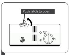
Press the release catch on the detergent dispenser to open the cover.
